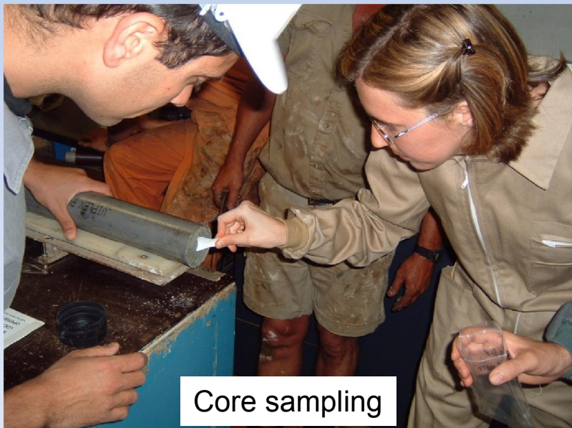
Recovery of the core liner from the piston coring system
