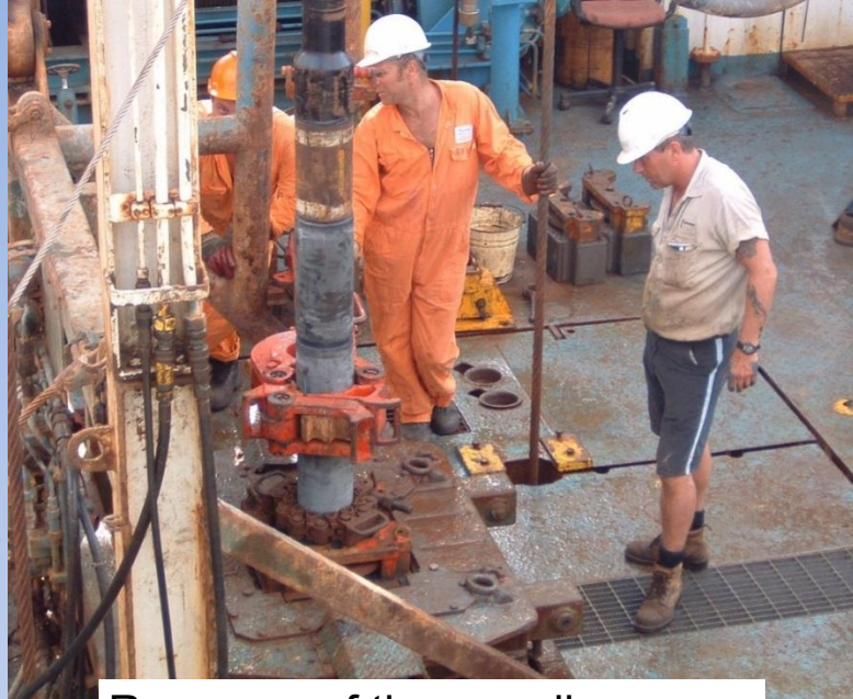
Recovery of the core liner from the piston coring system
